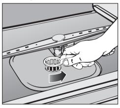
■ Turn the handle counterclockwise to release the triple filter system.
